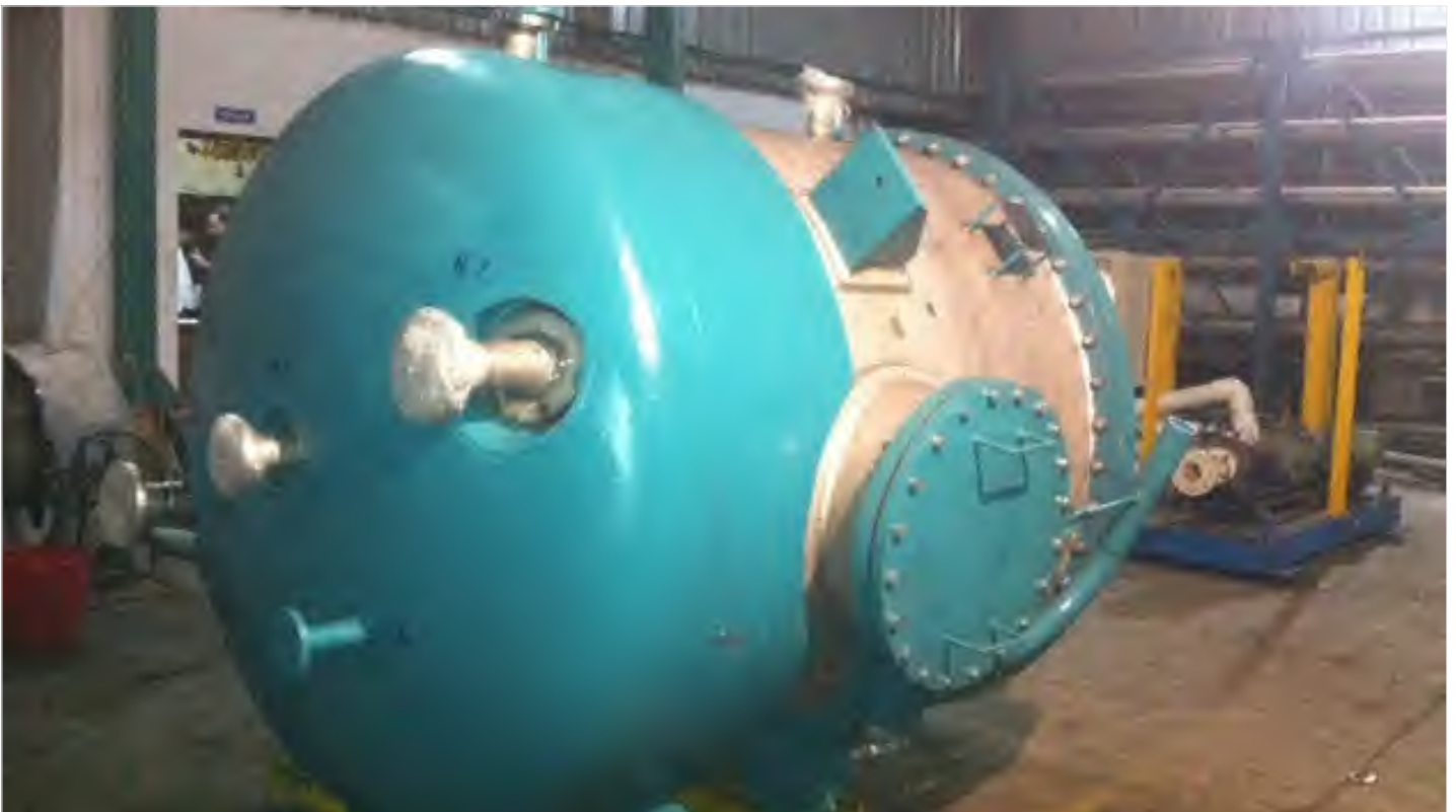
2,500 LTR Burger Vessel - Shell - SS304, Jacket - SA516GR70, Pressure - 8 Bar (G)
