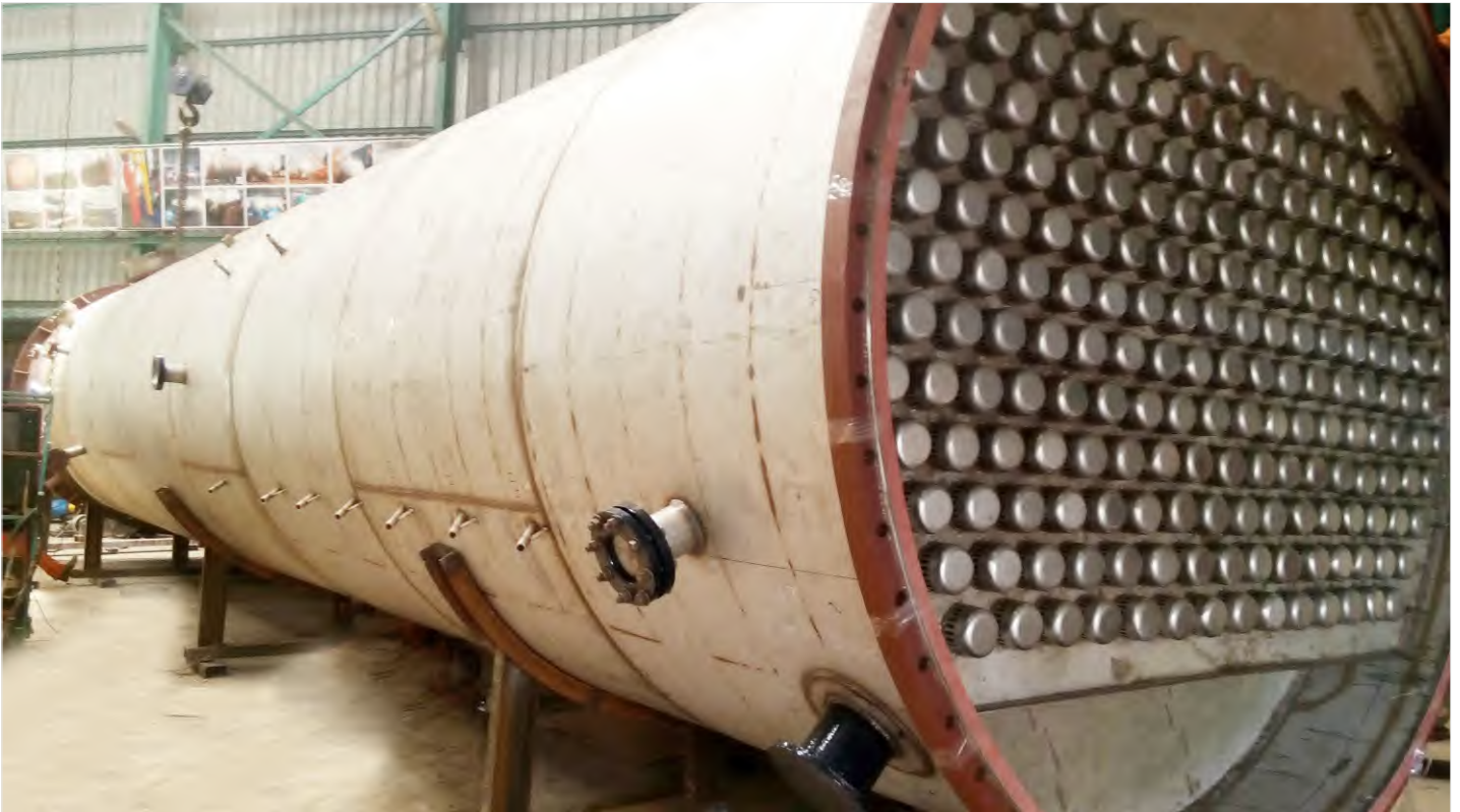
125 KLPD Distillery plant equipment : Rectifier Column
