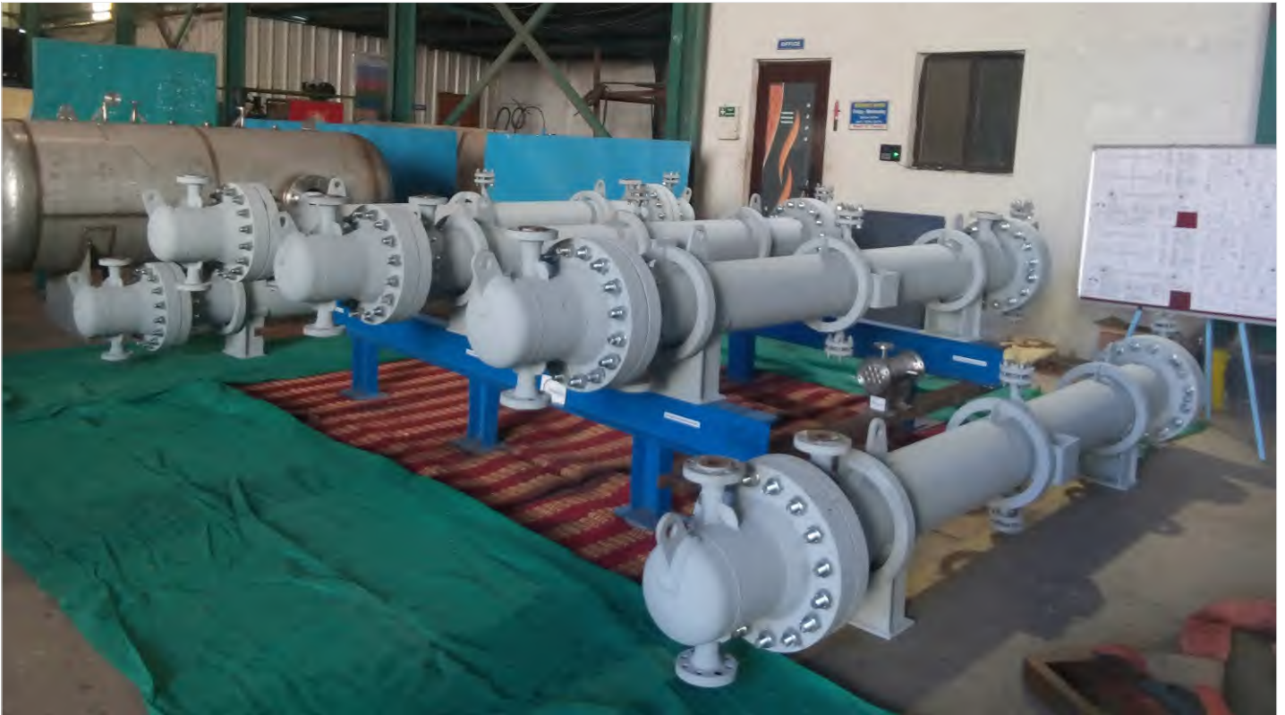
ASME "U" designator : Gas to Gas Exchangers, Pressure 62 Kg/Sq.cm
