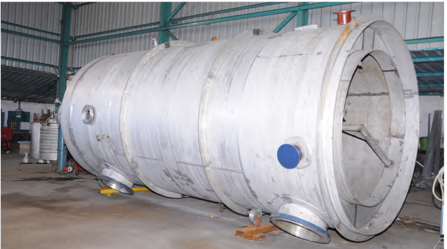
CDS Plant Equipment : Diameter 3 meter ,SS316L , Pack Column
