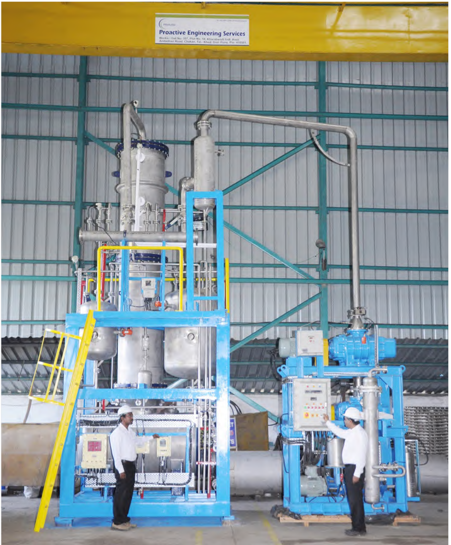
Mint Oil separation distillation plant along-with Dry vacuum system manufactured and supply at Melbourne Australia, successfully installation & commissioned the system.
