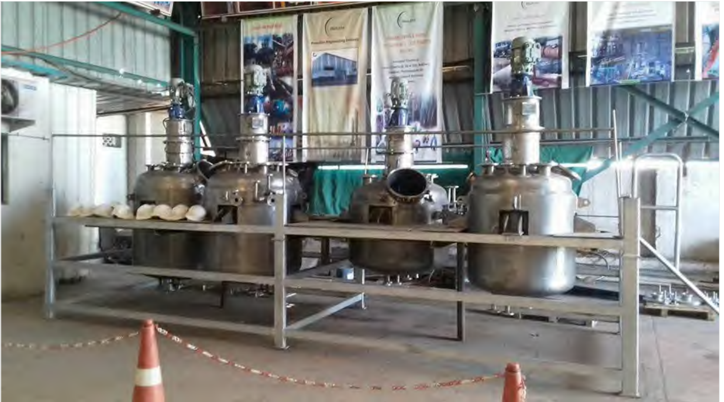
API equipment for Pharmaceutical chemicals : SS316 GMP Reactors
