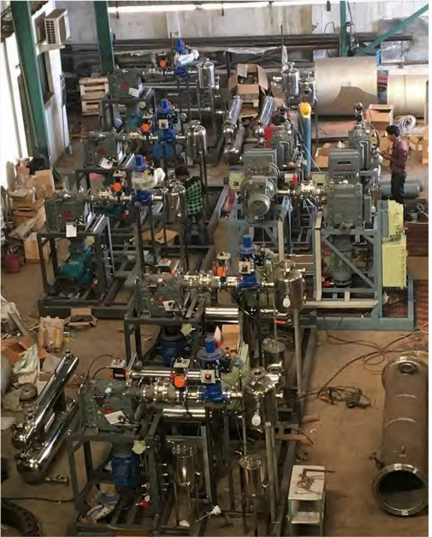
Dry Vacuum Skid mounted systems, under assemble condition
