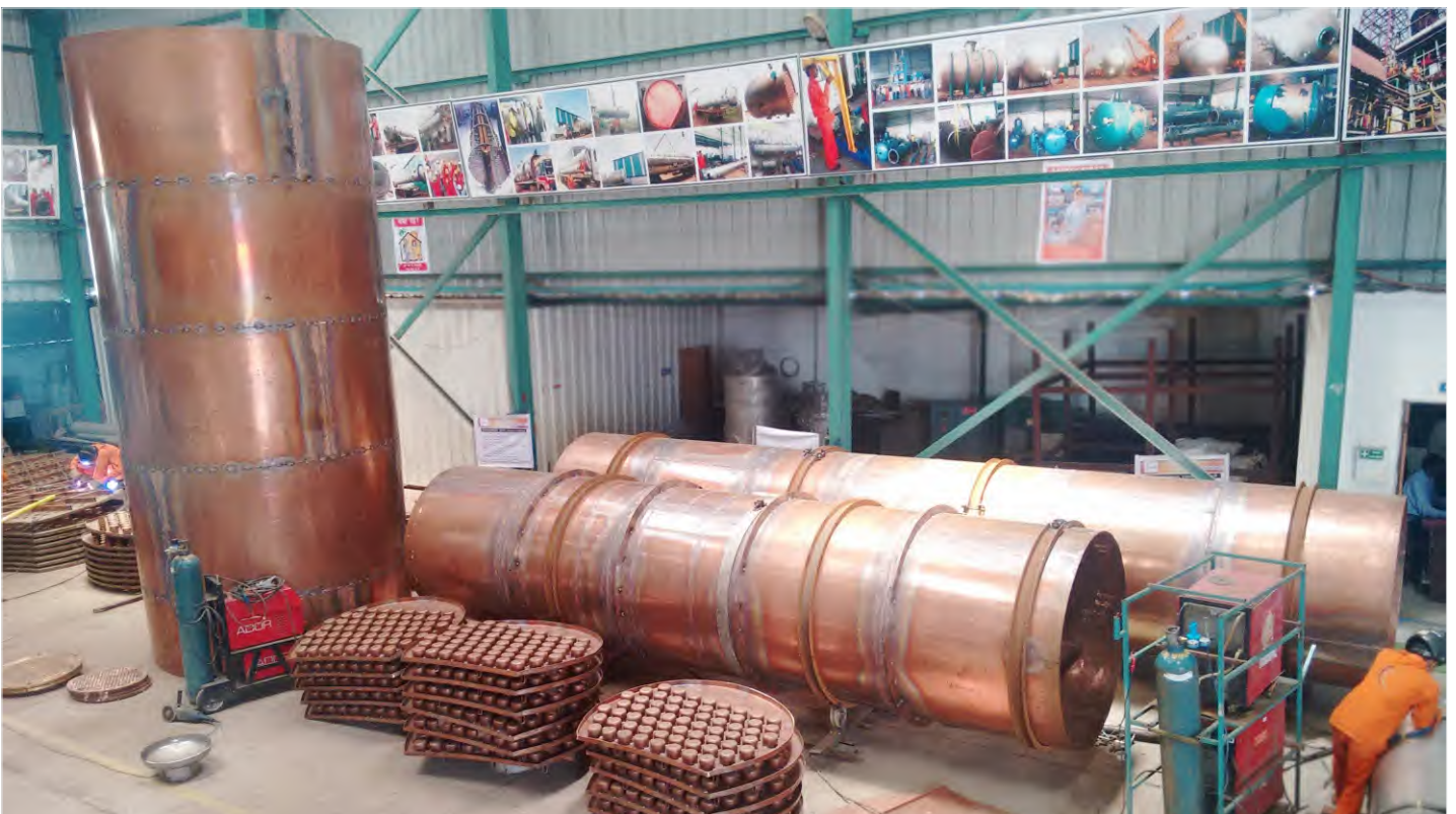
125 KLPD Distillery Plant Equipment : Refining column and bubble cap trays
