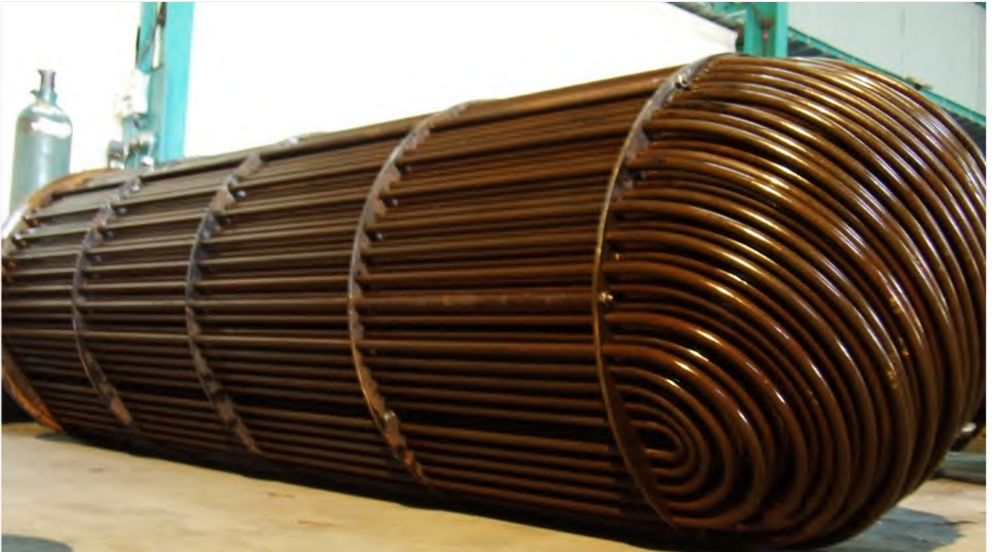
U tube Bundle For 90 MT capacity Kettle
