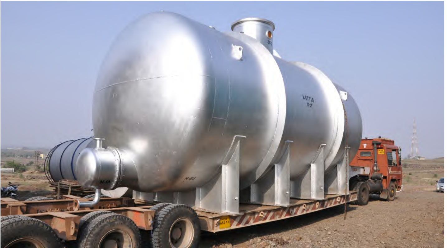
90,000 LTR Capacity Kettle - DIA. 4 MTR X 9.5 MTR Long
