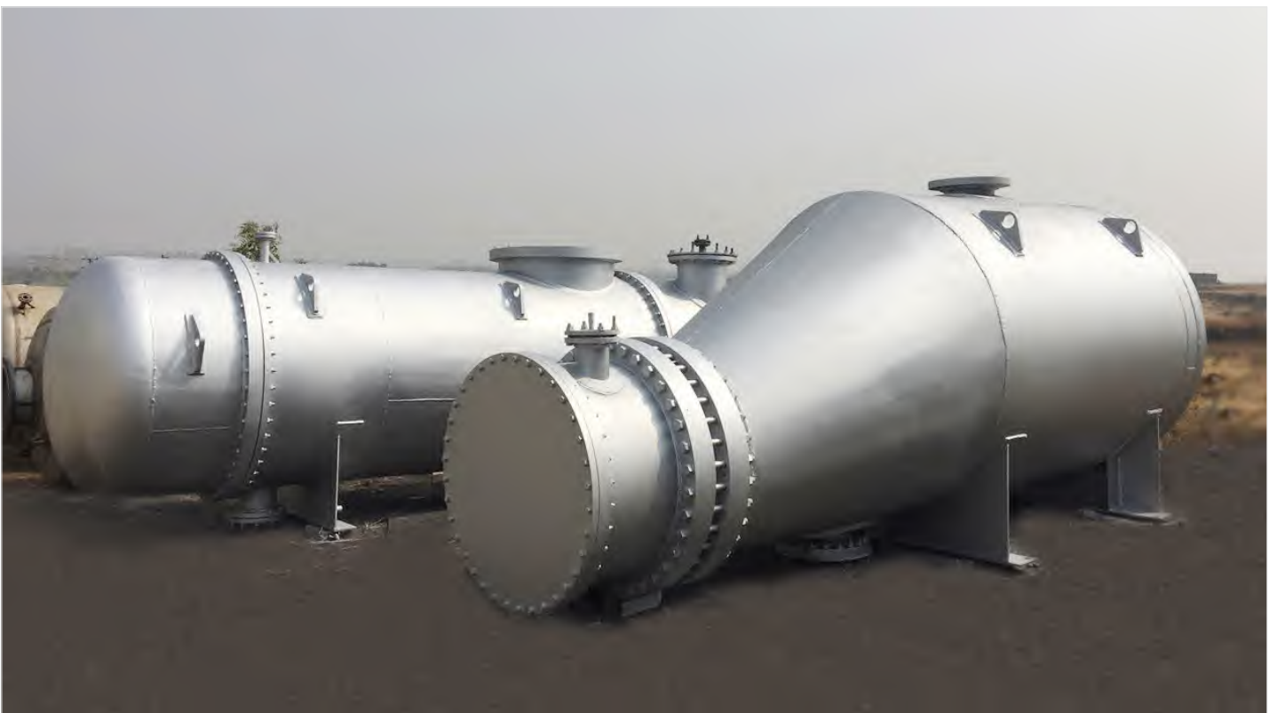
Power sector equipment U tube bundle kettle for Cement plant at UAE
