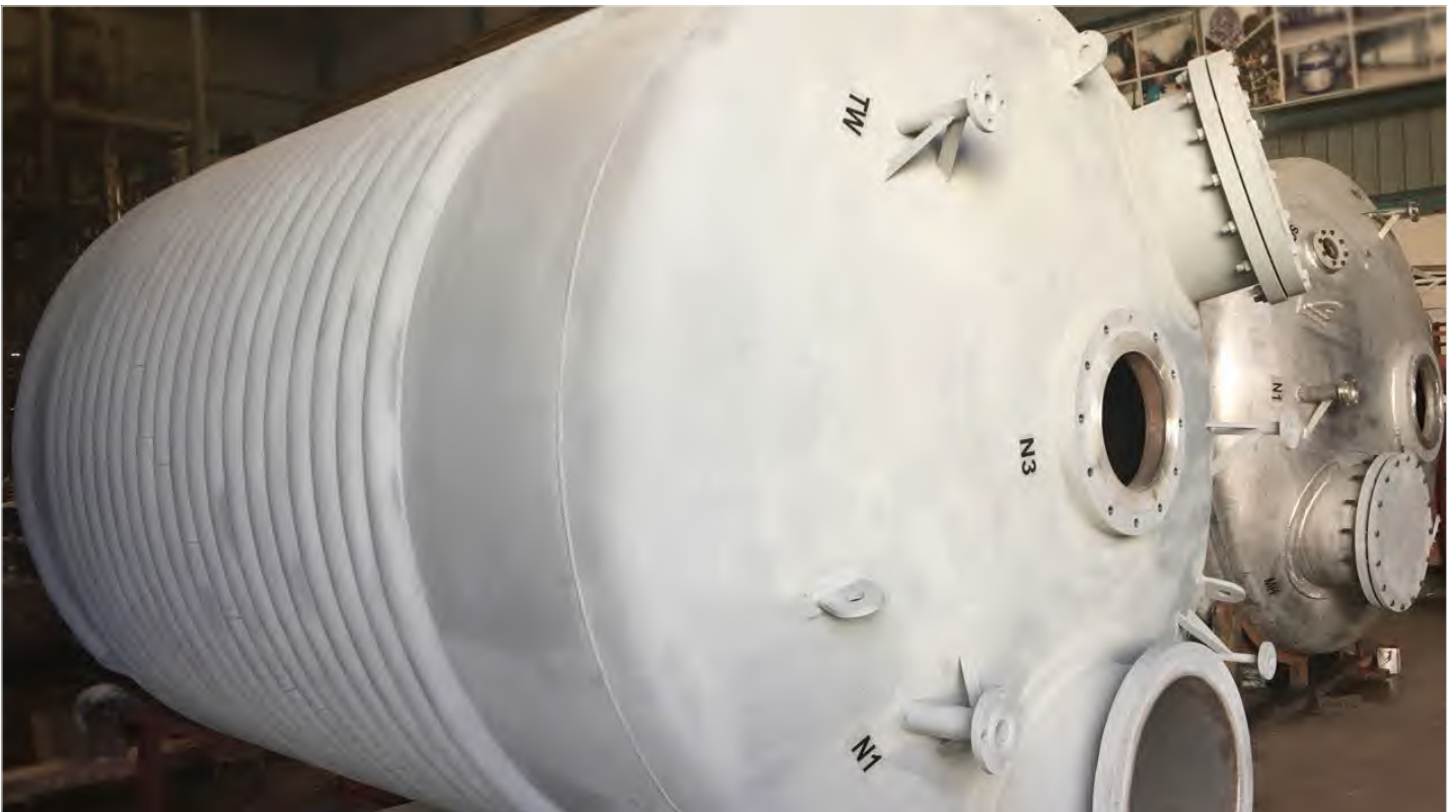
Limpet jacketed Reactors for Naphthalene Refining Plant
