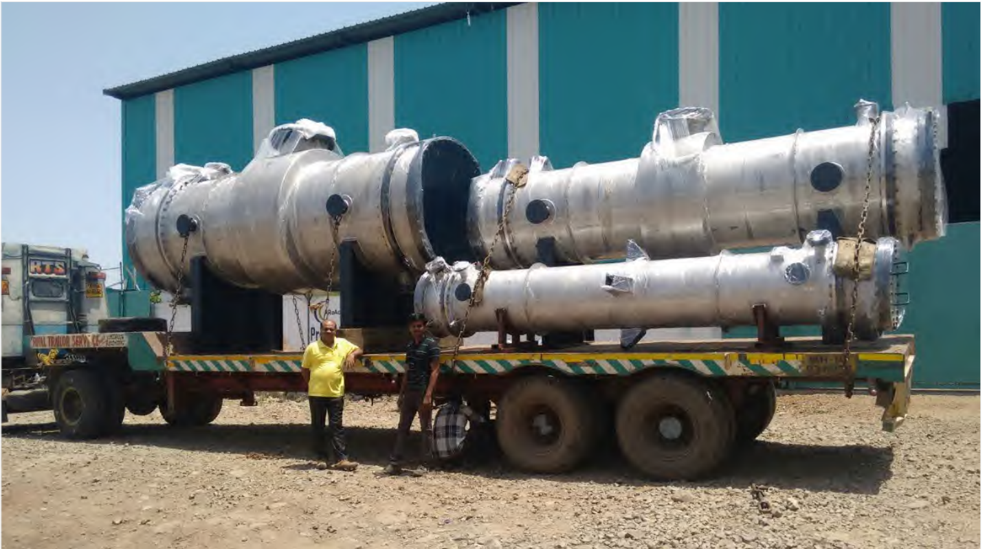
100 KLPD Distillery plant equipment : Reboiler and condensers
