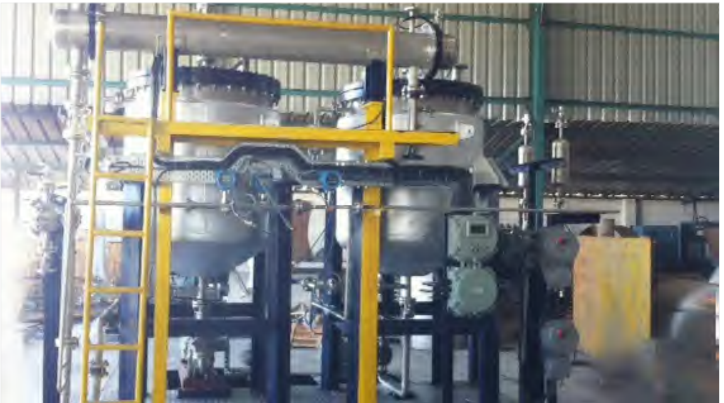
Modular Skid System for nitration at fertilizer chemical plant
