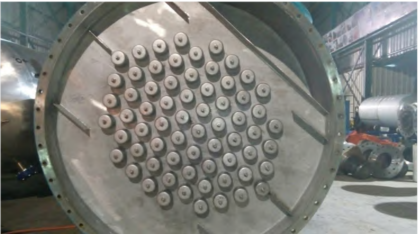
Internal Bubble cap tray - Distillation Column
