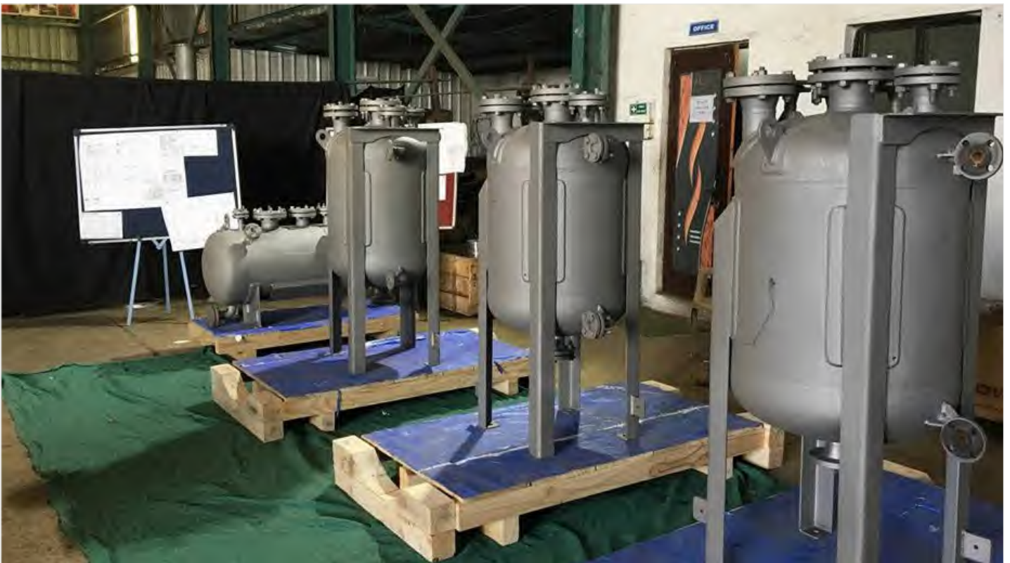
ASME "U" designator Expansion Tanks
