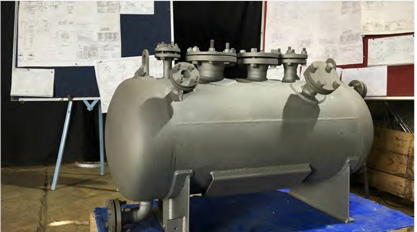
ASME "U" designator Pressure Vessel, Pressure 13.25 Kg/ Sq. cm
