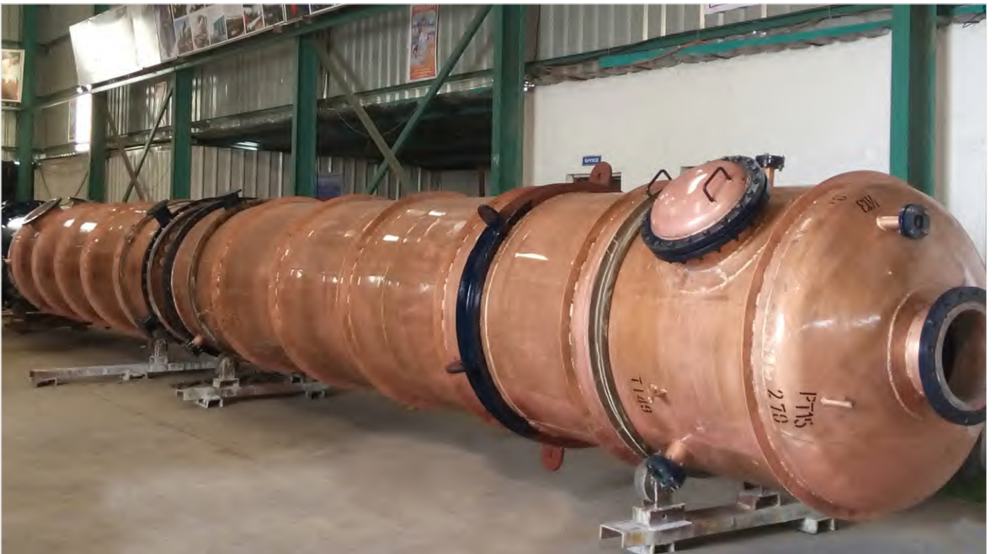
125 KLPD Distillery plant equipment : Refining Column under testing
