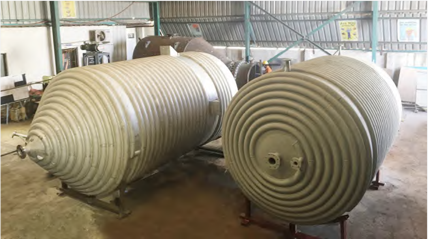
Limpet jacketed Reactors for Multiple Reactions Systems
